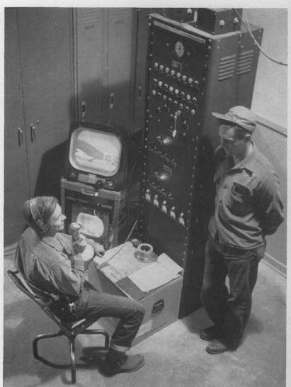
TEST CONTROL is maintained from this headquarters in the bunker which is well removed from the test track. Sid Cook, left, has direct communications with each work area along the track. Paul Syroid is engineer in charge of the test area. The two television screens show what is going on in the areas of the sled and the target.
